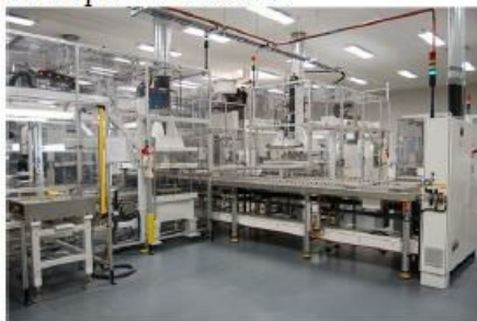
Figure Z : Example of fully automated MEA production line
